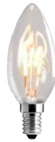
L200 LED SOFT FILAMENT CROWN Clear | W 3,5 D 3,5 H 10 | 10 pcs E14 | 2200K | 150 lm 3W (≈30W) | Dimmable
